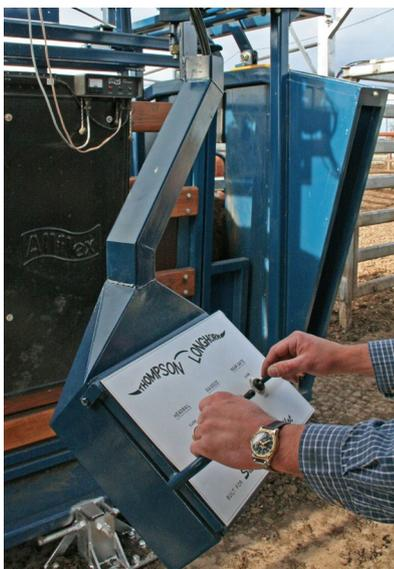
Operating console for a pneumatically-operated crush.
